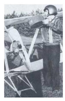
Mix of 100-octane gasoline and synthetic oil fuels the little engine. Moody reports no plug fouling with this mixture. Special 28-inch-diameter prop has very low pitch.
